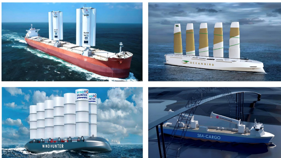
Figure 1. Typical engineering applications of modern Wind-Assisted Propulsion Systems (WAPS) on commercial ships. (Image from [1]).
