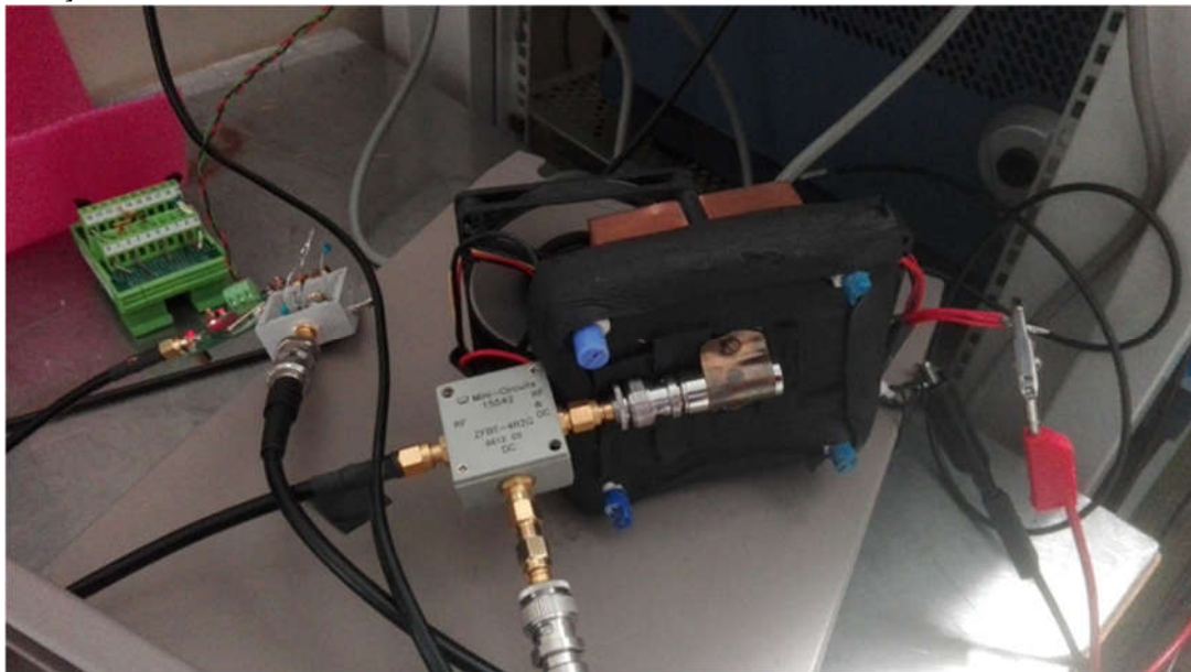
Figure 7. Laboratory test to evaluate the effect of decreasing the temperature of MCT detector by applying a Peltier's cell.
