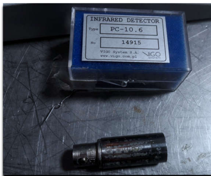
Figure 9. VIGO PC10.6 photoconductor with BNC female package.
