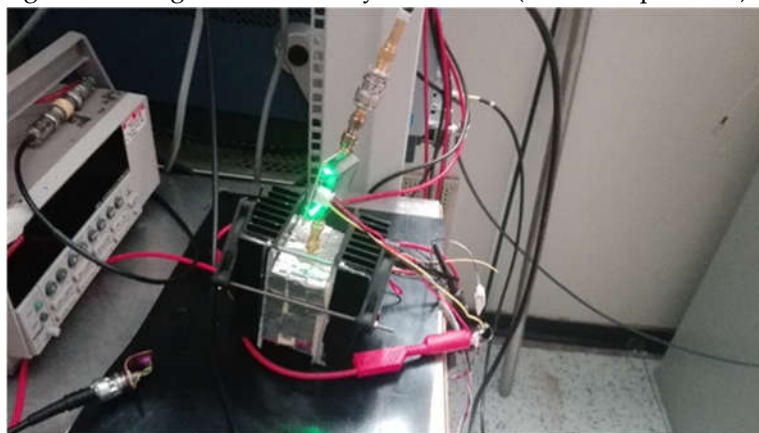
Figure 12. The Hamamatsu detector between two Peltier cells.
