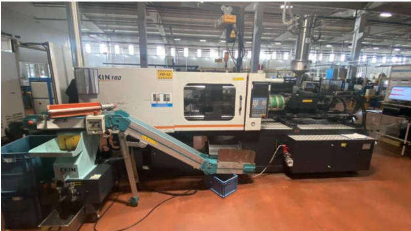
Figure 7. Horizontal plastic injection molding machine used for the trials.
