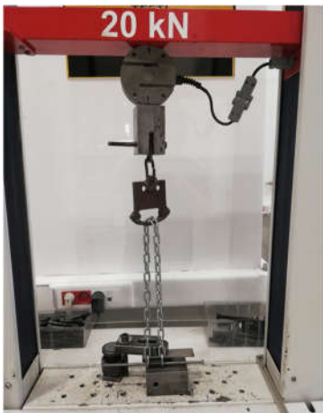
Figure 9. Attachment of the slide lock to the tensile testing machine.
