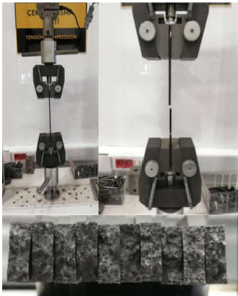
Figure 3. Application of the tensile test and visuals of the fracture surfaces on the 20kN capacity testing device of Kalitest Machine.
