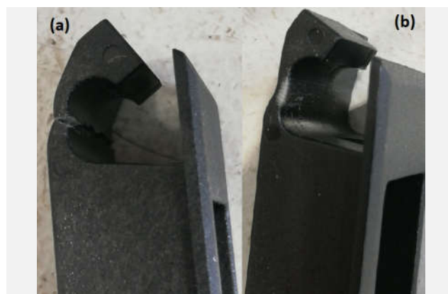
Figure 10. Images of the tensile test results of the 10% olive seed-filled ABS product from the 1st trial (a) and the samples from the 6th trial produced with standard ABS raw material (b) after the tensile test.
