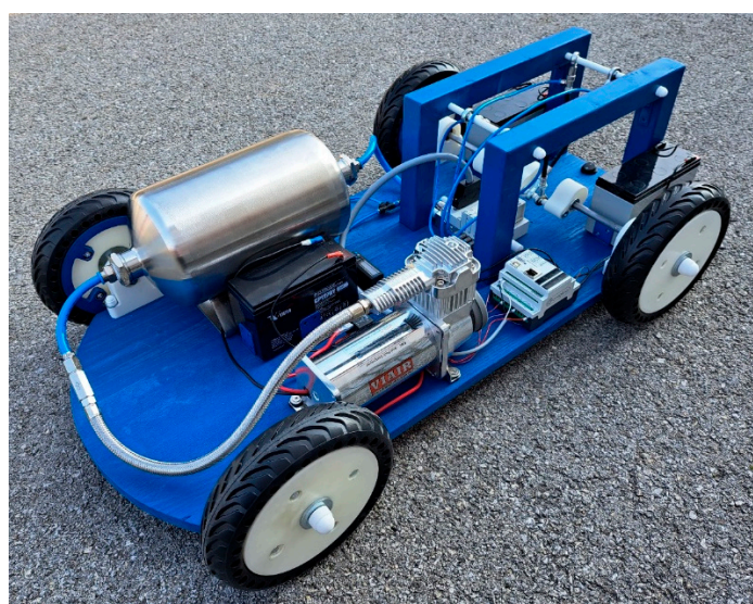
Figure 7. Vehicle with pneumatic muscle engine.
