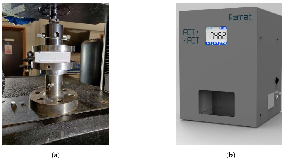
Figure 4. Edge crush test: (a) Universal Testing Machine (Instron 5569); (b) FEMAT lab. device.
