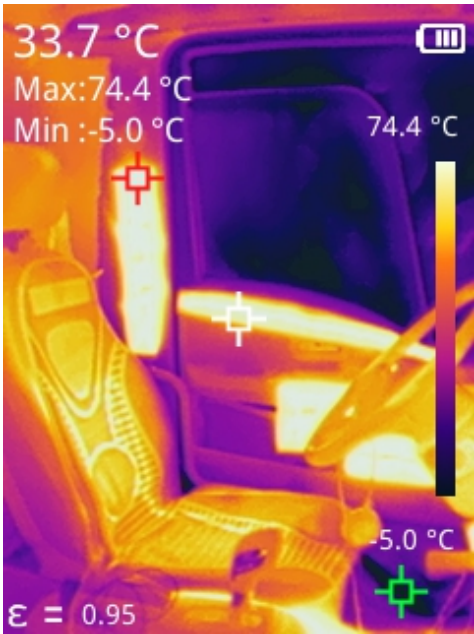
Figure 3. Thermal camera image showing localized heating around the driver and seat, enabled by integrated heating panels.
