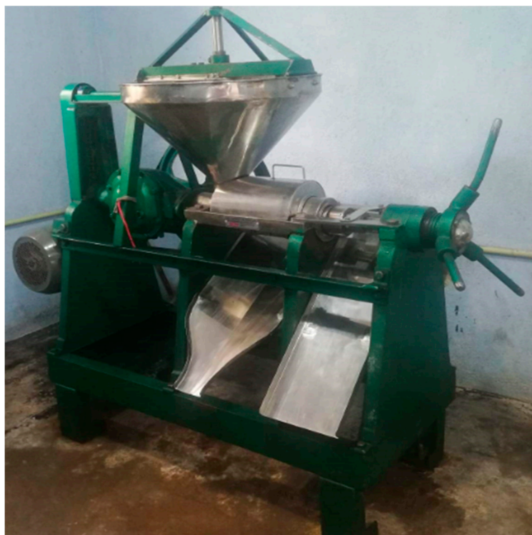
Figure 10. The screw type expeller.
