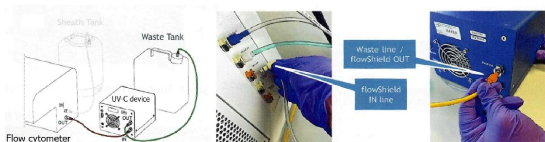
Figure 1. Schematic and representative image showing how the UV-C flow shield device is connected to the waste tank of the flow cytometer. Images are adopted from A.P.E flowShield User Manual [9].
