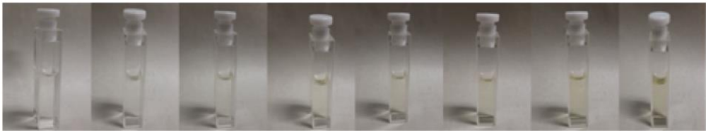
Figure 5. Colorimetric studies of receptors of I (7.88 mM) with aliquots 0.4 mM copper (II) ions.
