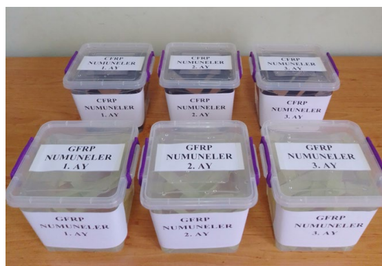
Figure 11. Soaking GFRP and CFRP samples in sea water for 1, 2 and 3 months for three-point bending.
