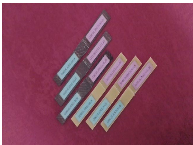
Figure 8. Visual observation of the surface morphology of GFRP and CFRP specimens prior to the four-point bending test.
