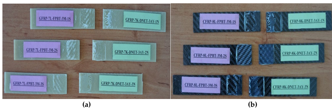
Figure 25. Views of GFRP-7L-FPBT-3M specimen (a) and CFRP-8L-FPBT-3M specimen (b) after four-point bending test.
