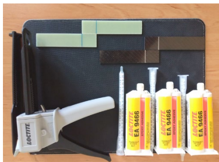
Figure 6. Bonding Process of GFRP and CFRP Specimens Using Loctite Hysol-9466.
