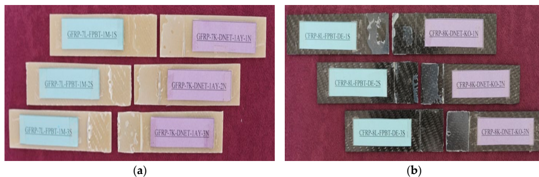
Figure 22. Views of the GFRP-7L-FPBT-DE-1S specimen (a) and CFRP-8L-FPBT-DE-1S specimen (b) after the four-point bending test.
