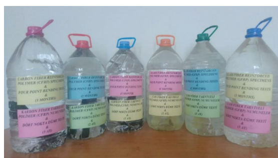
Figure 12. Soaking GFRP and CFRP samples in sea water for 1, 2 and 3 months for four-point bending tests.
