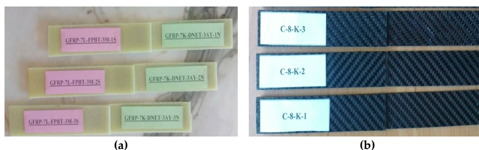
Figure 10. GFRP (a) and CFRP (b) specimen configurations used during the four-point bending test.
