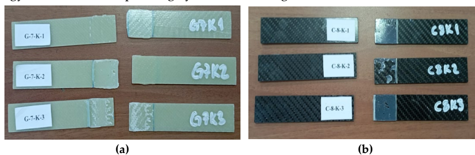
Figure 16. Views of the G-7-K sample after the three-point bending test (a) and the C-8-K sample after the test (b).
