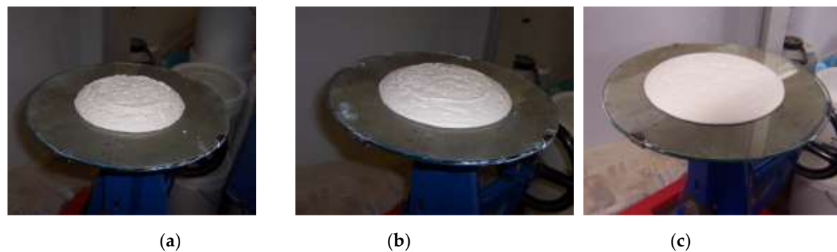
Figure 9. Samples of coarse mortar (a), fine plaster (b) and finishing plaster (c) after the mold lift during the spreading test.
