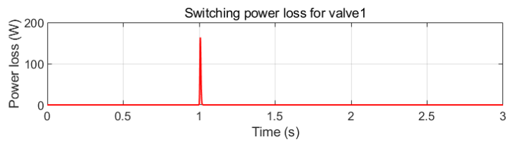
Figure 18. Switching power loss of HS system.
