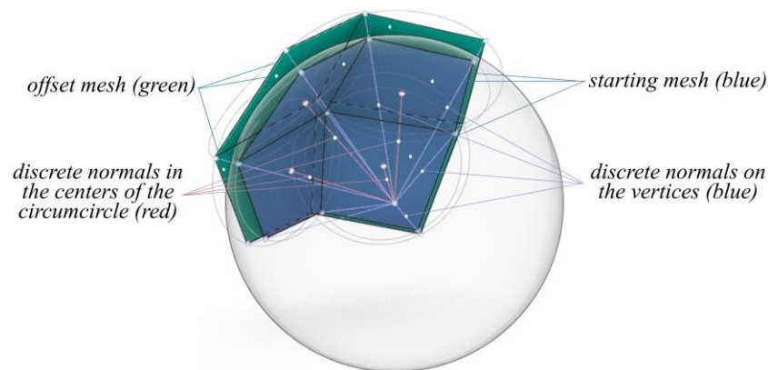
Figure 2. Display of the two sets of discrete normals of the circular mesh system on the unit sphere (Tošić et al. 2020).
