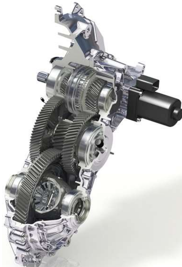
Figure 6. Two-speed gearbox with a forced-synchromesh mechanism [2].
