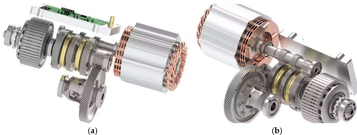
Figure 8. Three-speed gearbox from Ricardo engineers [8].
