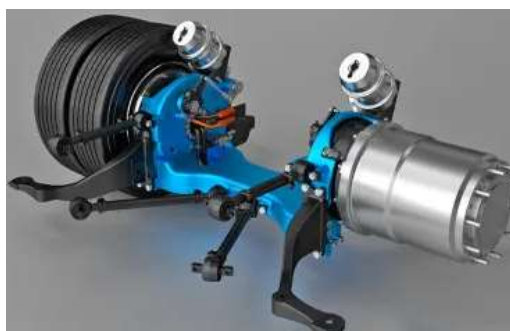
Figure 15. Planetary wheel hub drives for heavy-duty trucks and buses [14].
