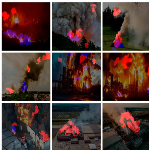
Figure 41. Applying LIME XAI for feature/area contribution importance on nine images using YOLOv10n.
