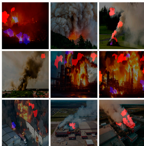
Figure 39. Applying LIME XAI for feature/area contribution importance on nine images using YOLOv5nu.
