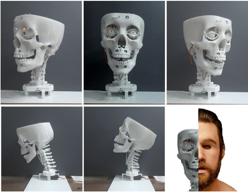
Figure 2. Arslan’s Physical Structure and neck rotations [1].
