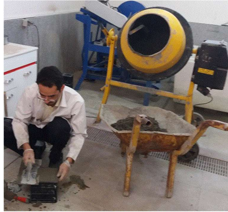
Figure 2. The process of concrete production: mixing and pouring.
