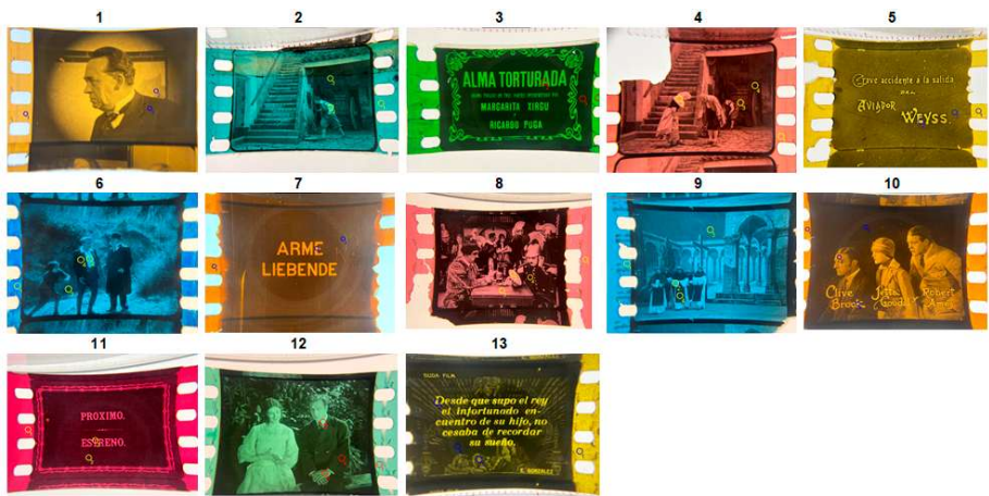
Figure 1. Images of the 13 frames from early films considered in this paper (see Table 1). We have added the small numbered circles in the frames to indicate the specific regions where spectral transmittances were measured (see main text). The colors in this Figure are only approximate.
