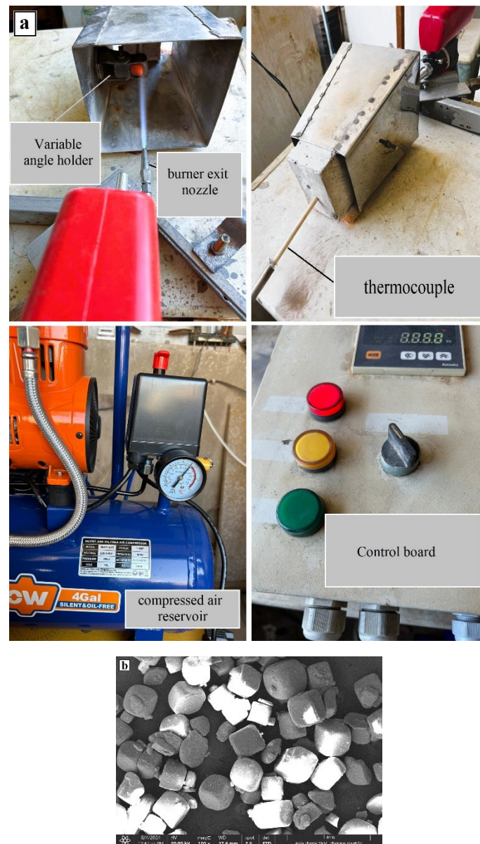
Figure 5. a) Air jet hot solid particle erosion test, b). Silica erodent powder used for SPE test.
