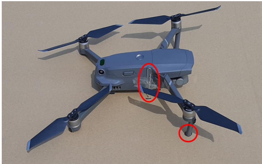
Figure 4. The DJI Mavic 2 Pro used for the measurements, with necessary markings on the landing platform and the paperclip marker used to indicate the landing points.
