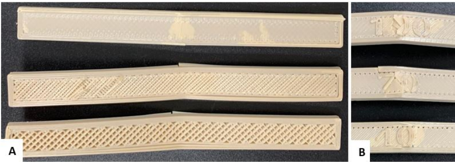
Figure 15. Flexural test specimens: A - Cross section of the specimens to visualize the filling density. B - Flexural failure of the standardized specimen with filling levels of 40%, 70%, and 100%.
