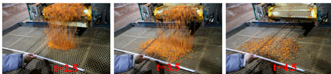
Figure 16. Experimental prototype of variable-amplitude vibrating screen.
