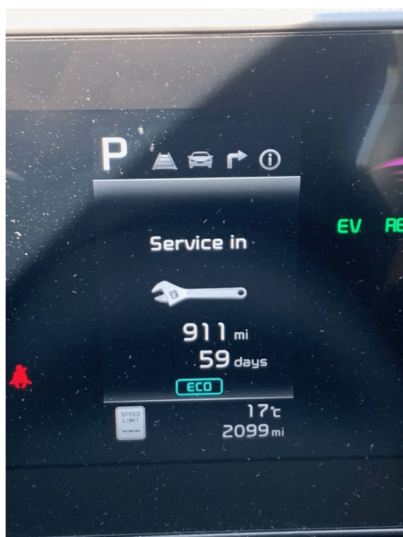
(a) Conventional dashboard service reminder based on fixed mileage or time intervals.
