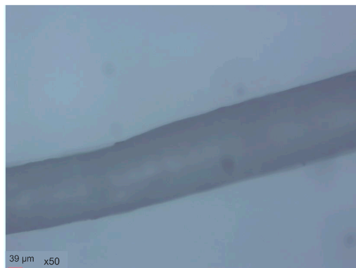
Figure 6. Optical microscope image of mango fiber treated with NaOH.
