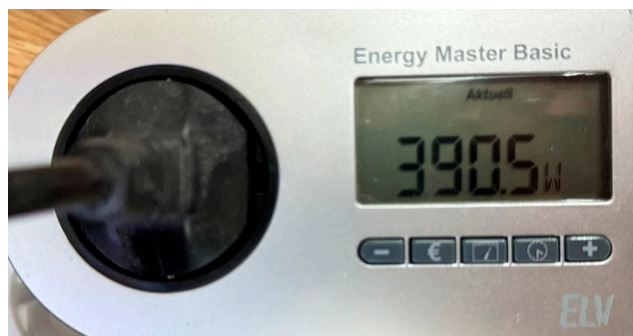
Figure 3. Power meter (ELV Energy Master): Measured minimum load: 390.5 W.
