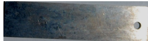
(b) After hanging, the surface is cleaned with acetone.
