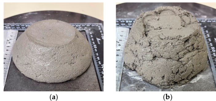
Figure 8. Appearance of mortar during 15-stroke flow test. (a) immediately after mixing. (b) after 30 min of mixing.
