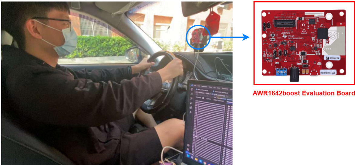
Figure 12. Deployment of the radar devices within the vehicle.
