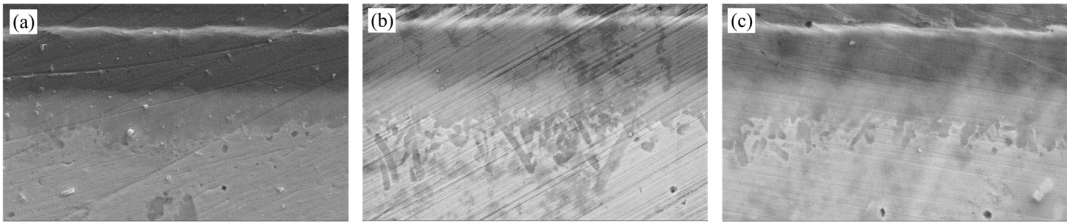
Figure 10. State of IMCs after aging in argon atmosphere.
