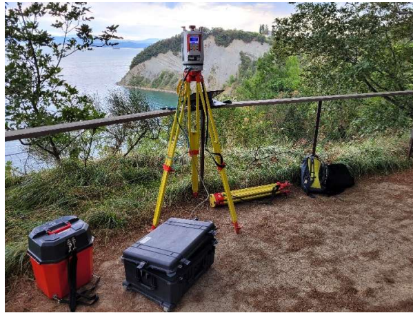
Figure 4. TLS setup overlooking the selected section of the cliff.
