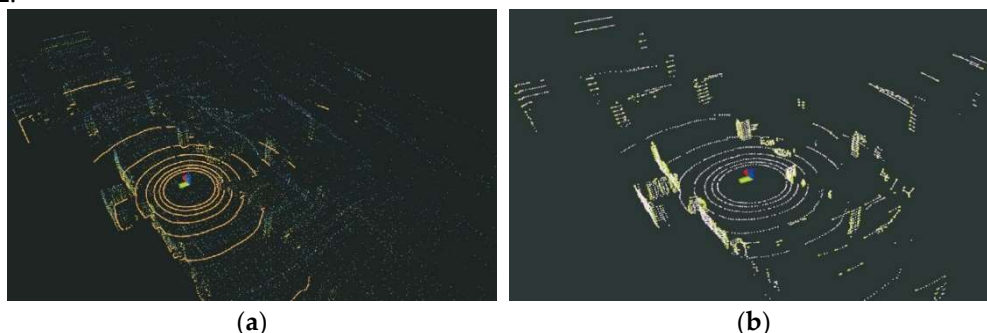
Figure 2. (a) Point cloud data obtained by lidar; (b) The extracted edge and plane features.
