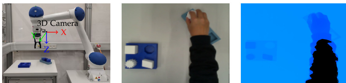
Figure 9. (a) Demonstration setup; (b) Color image; (c) Aligned depth image
