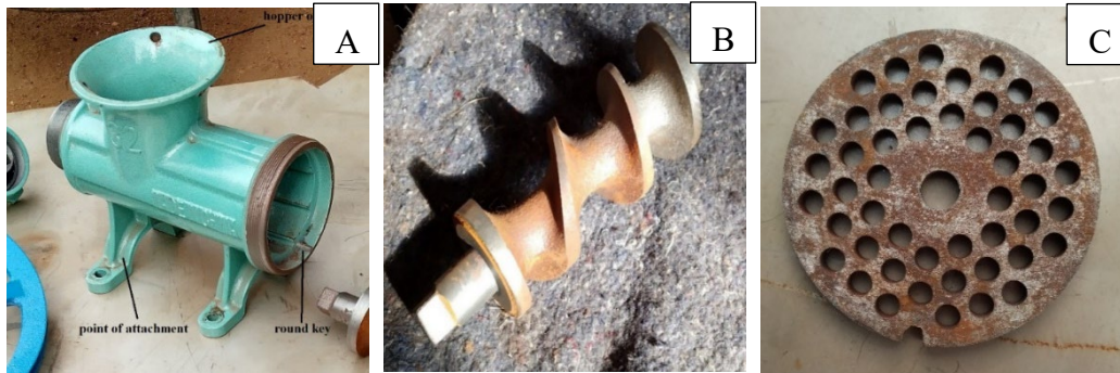
Plate 1: Parts of the existing pelletizing machine; (A) compression chamber (B) Auger of the pelletizing unit (C) pelletizing die.
