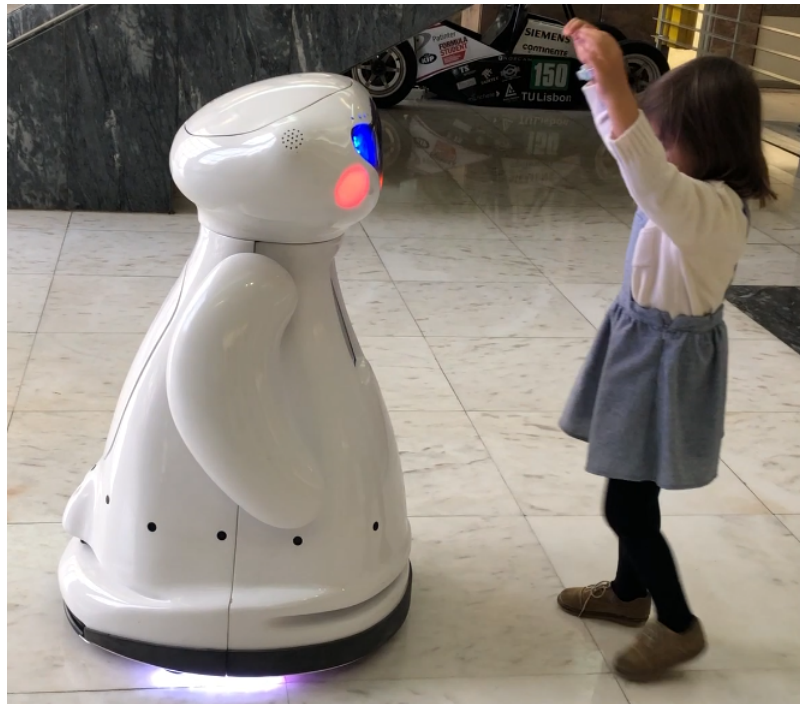
Figure 3. Child interacting with a social robot. Wizard of Oz experiment using a Mbot robot. The wizard controlled only the speech interaction. The motion of the robot was autonomous, and the interaction with the motion of the child resulted similarly to a dance.
