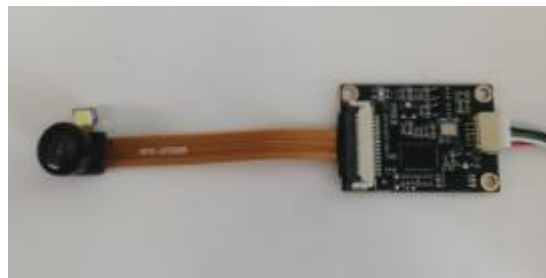
Fig. 3. USB Camera Module 2 Megapixel 60
