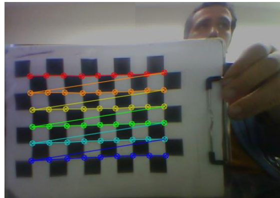
Fig. 7. The process of finding the corners of a checkerboard
