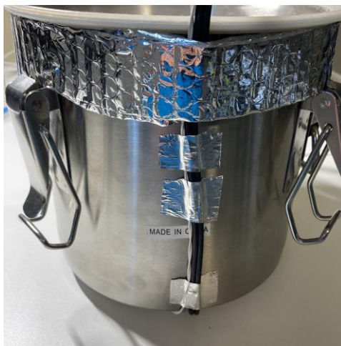
Figure 5. If installed, the heater power cable and sensor wires may be fed up the wall of the chamber for strain relief, but this is not required.
