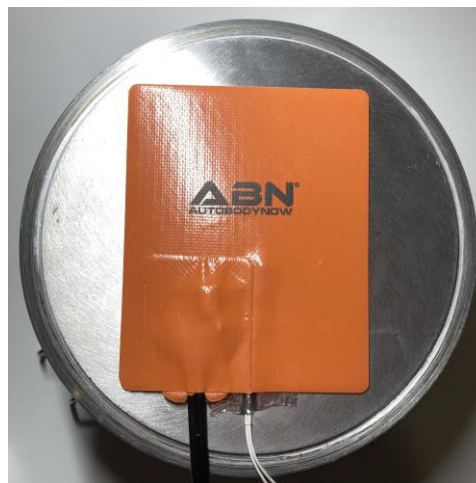
Figure 10. The heating element was adhered to the base of the chamber, with the thermistor secured on the interface.
