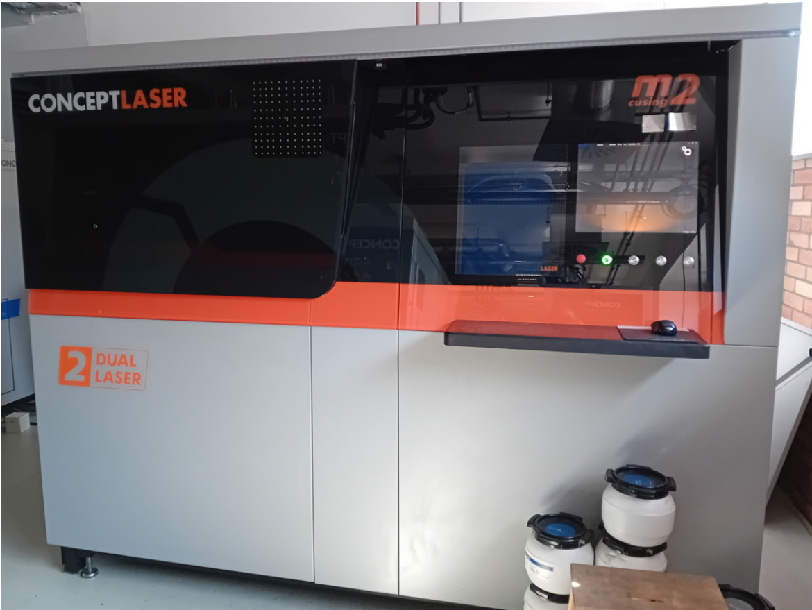
Figure 1. The image above depicts the powder bed fusion printer used to print steel specimens.
