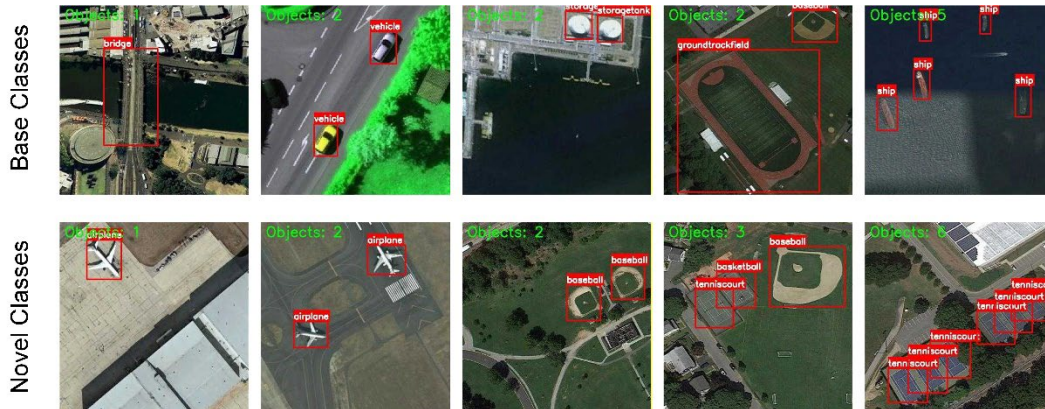
Figure 5. Visualization of detection results in the 10-shot experiments on the NWPU VHR-10.v2 dataset under Class Split 1. The first row presents examples from the base classes, while the second row presents examples from the novel classes.
