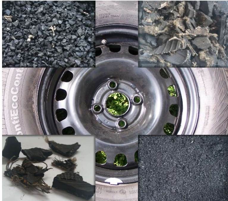
Figure 3. Examples of various tire rubber waste used in geoengineering applications (source: photo of M. Jastrzębska).
