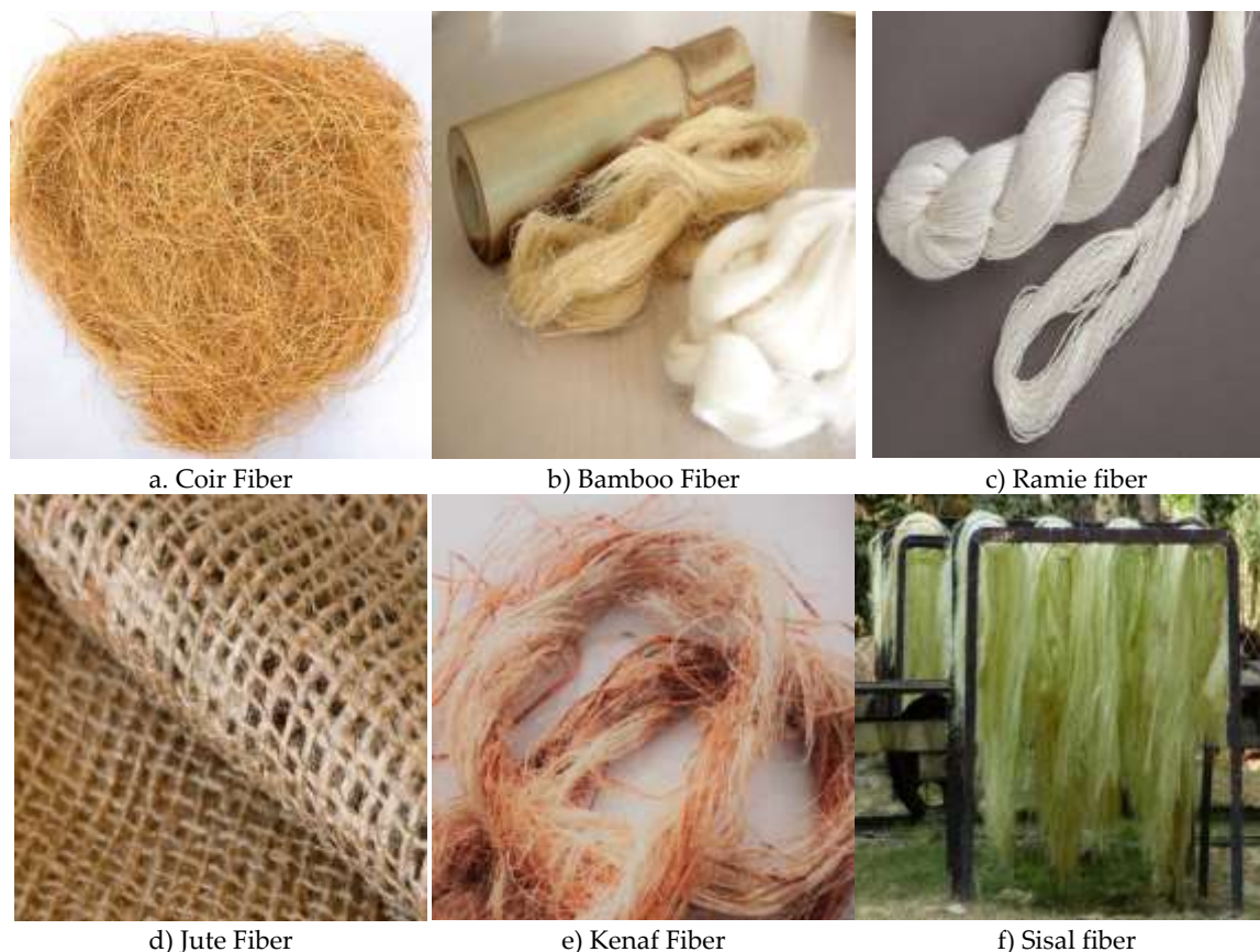
Figure 1. Natural fibres a) coir fibre [29], b) bamboo fibre [30], c) ramie fibre [31], d) jute fibre [32], e) kenaf fibre [33] and f) sisal fibre [34].
