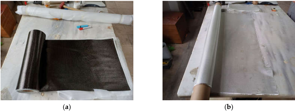
Figure 3. FRP types: (a) CFRP, (b) GFRP.
