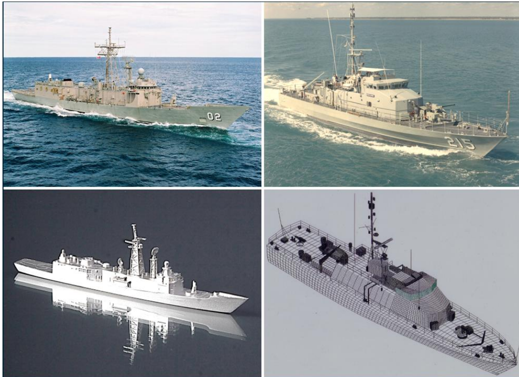
Figure 7. The upper left image shows the FFG 7 while that on the upper right shows the Fremantle Class Patrol Boat. The lower left images shows the scale model FFG-7 sitting on the aluminum ground plane that represents the smooth sea surface, while that on the lower right shows the digital wire model used for the NEC 4 calculations.
