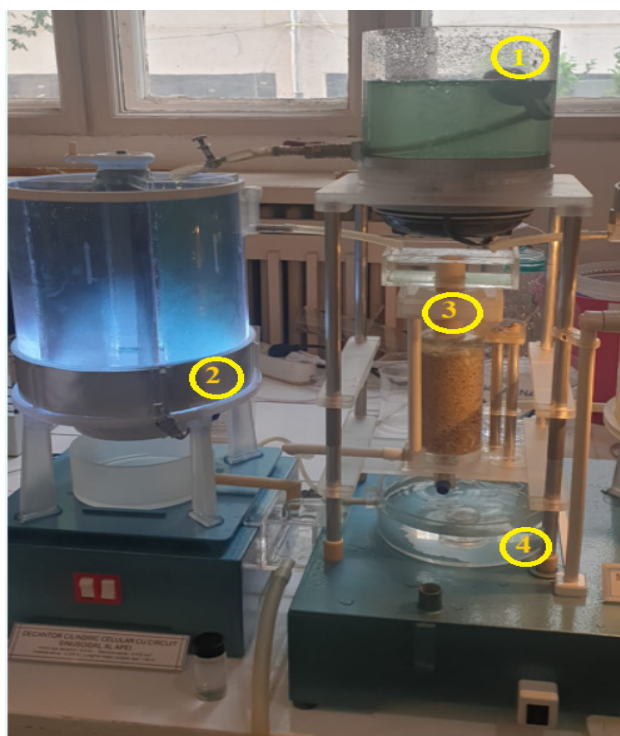
Figure 1. Microplastics decantation and filtration installation.
