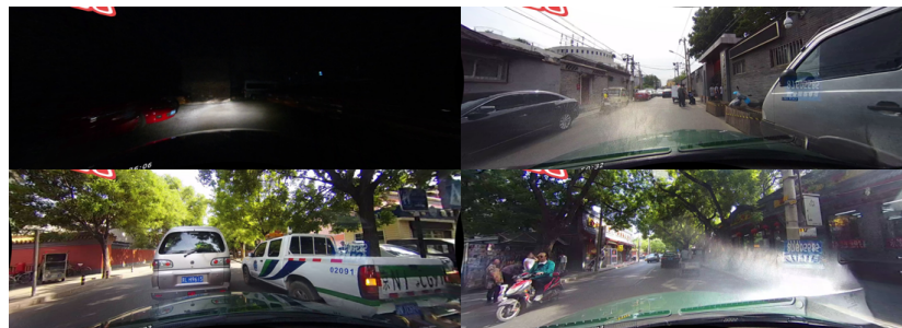
Figure 1. Corner cases in lane detection. There are many challenging scenarios in the lane detection task, such as at night, with severe occlusions, resulting in no visual clues for visual task.
