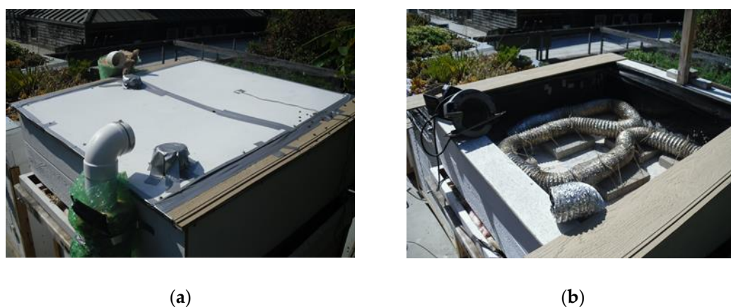
Figure 7. Experimental testing unit with a roof pond sealed by an aluminum sheet (a); detail of the WAHE (b).
