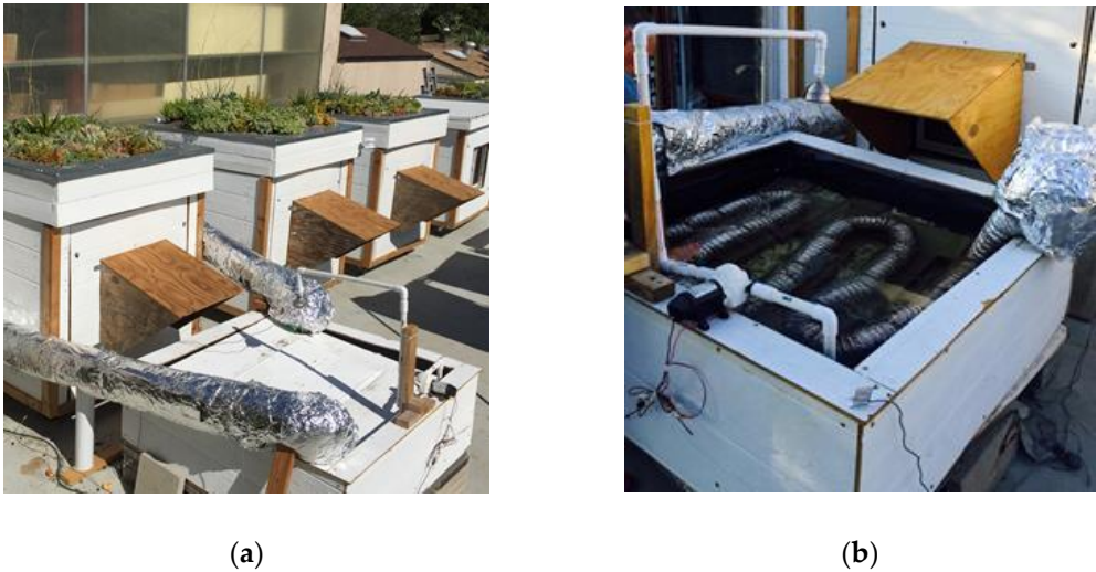
Figure 5. Green roof connected to a WAHE (a); detail of the WAHE (b).
