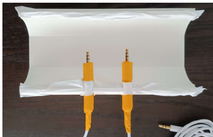
Figure 20. Ear-EEG phantom assembly - antennas and railing fittings were sealed with tape
