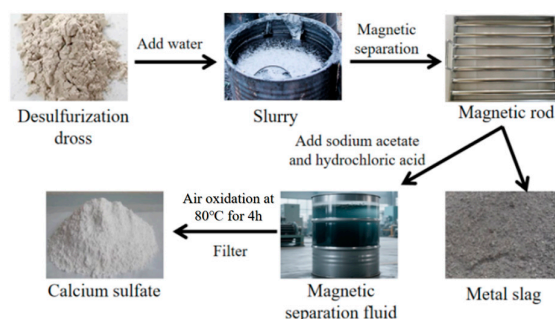
Figure 13. Process of preparing high value-added calcium sulfate from desulfurization dross [80].
