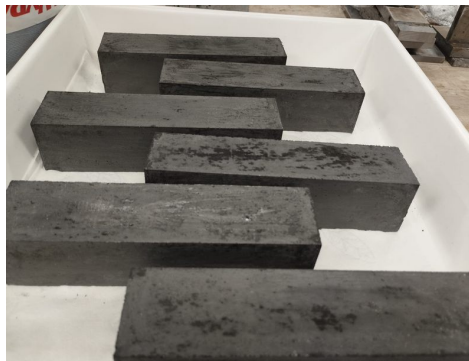
Figure 3. Demolded Aachen GP prismatic specimens ( 40 \times 40 \times 160 mm) prior to curing used for flexural strength testing
