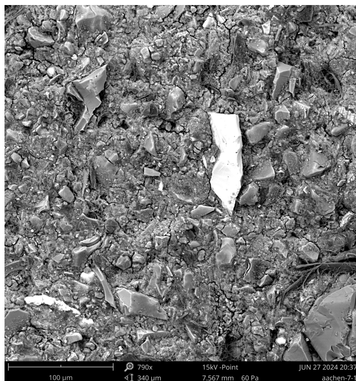
Figure 16. SEM micrograph of Aachen GP at 28 days (790 \times ) showing large, irregular, and interconnected pores with residual slag inclusions. The open pore structure indicates incomplete encapsulation by the gel, consistent with higher measured porosity and slower reaction kinetics.
