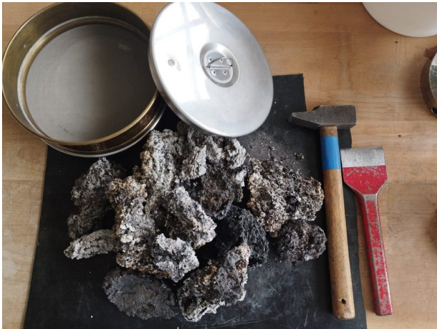
Figure 1. Coarse iron-rich slag as received from Siempelkamp (Germany), with typical particle sizes ranging from 5 cm to 20 cm.
