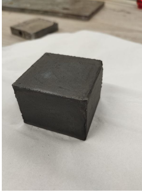
Figure 2. Demolded Aachen GP cubic specimen ( 40 \times 40 \times 40 mm) prior to curing used for compressive strength testing and other analysis.
