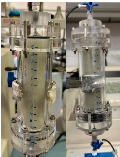
Figure 6. Visual comparison of the column before and after the BC@CMC breakthrough experiment.
