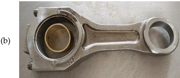
Figure 3. Connecting rod bushing (a) before and (b) after the push-out test.
