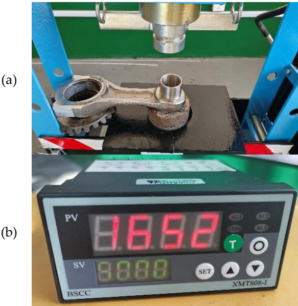
Figure 4. (a) Schematic of the push-out test setup; (b) Measured retention force for a bushing with 0.04 mm interference.
